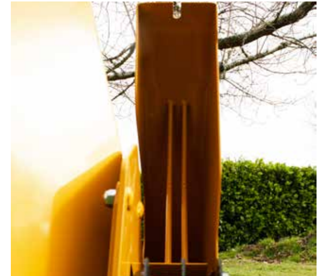
Fixed gate for consistent discharge control of fine mulch
